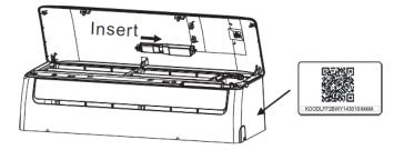
WARNING This interface is only compatible with SMART KIT(wireless module) provided by the manufacturer.
